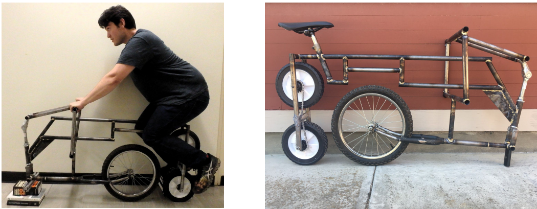
Figure 6. Fabricated bicycle with and without a rider seated in the optimal position. The front end is supported by a stack of books in the left photo, but this is replaced with a swiveling caster when riding.
