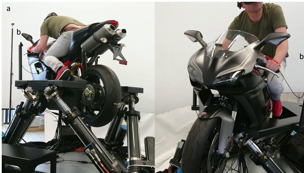
Figure 2. The Cruden motorcycle simulator consisting of a Ducati 848 evo motorcycle mock-up mounted on a Stewart 6-DoF motion platform. Visualization of the virtual scenery by means of head mounted display (HMD).
