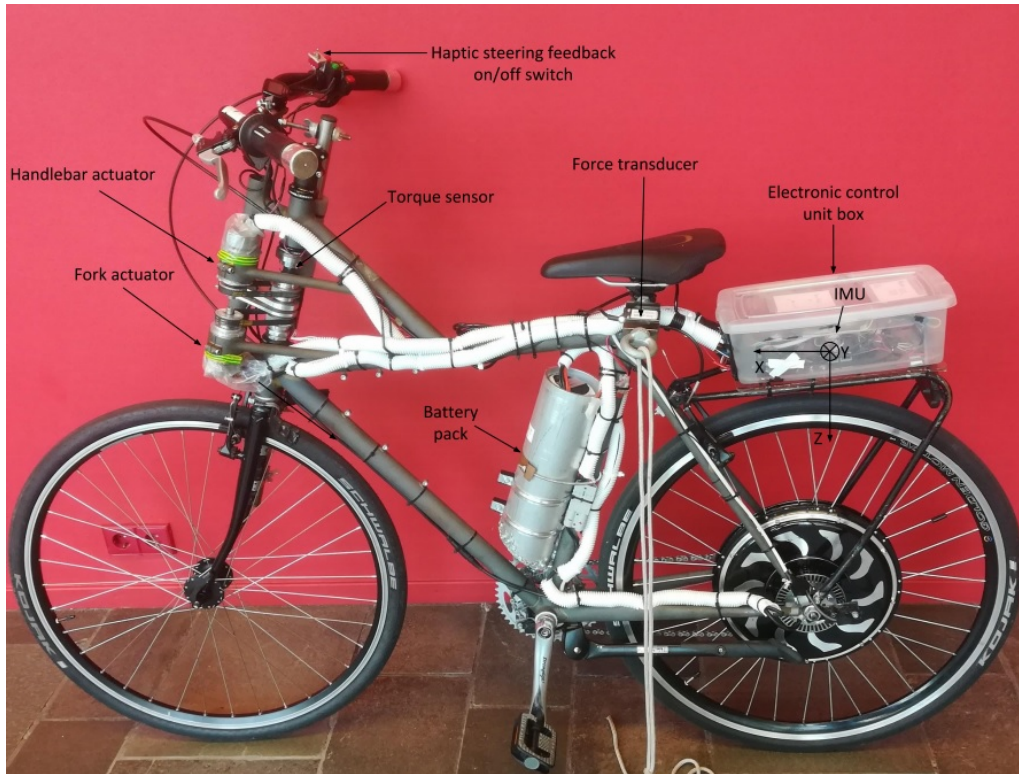
Figure 1: Prototype of the steer-by-wire bicycle with steering and handlebar actuators, sensors, digital controller and custom made battery pack.
