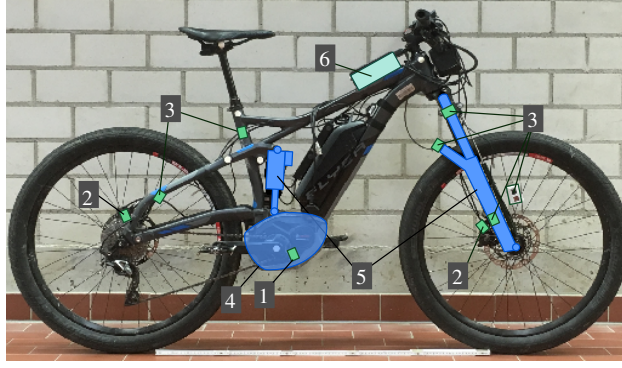
Figure 2. Test bike with measurement setup consisting of drive-integrated torque sensor (1), wheel speed encoders (2), inertial measurement units (3). Additionally, there is the electric drive (4) and semi-active dampers (5) as well as an electronic control unit (6) for logging and prototyping.
