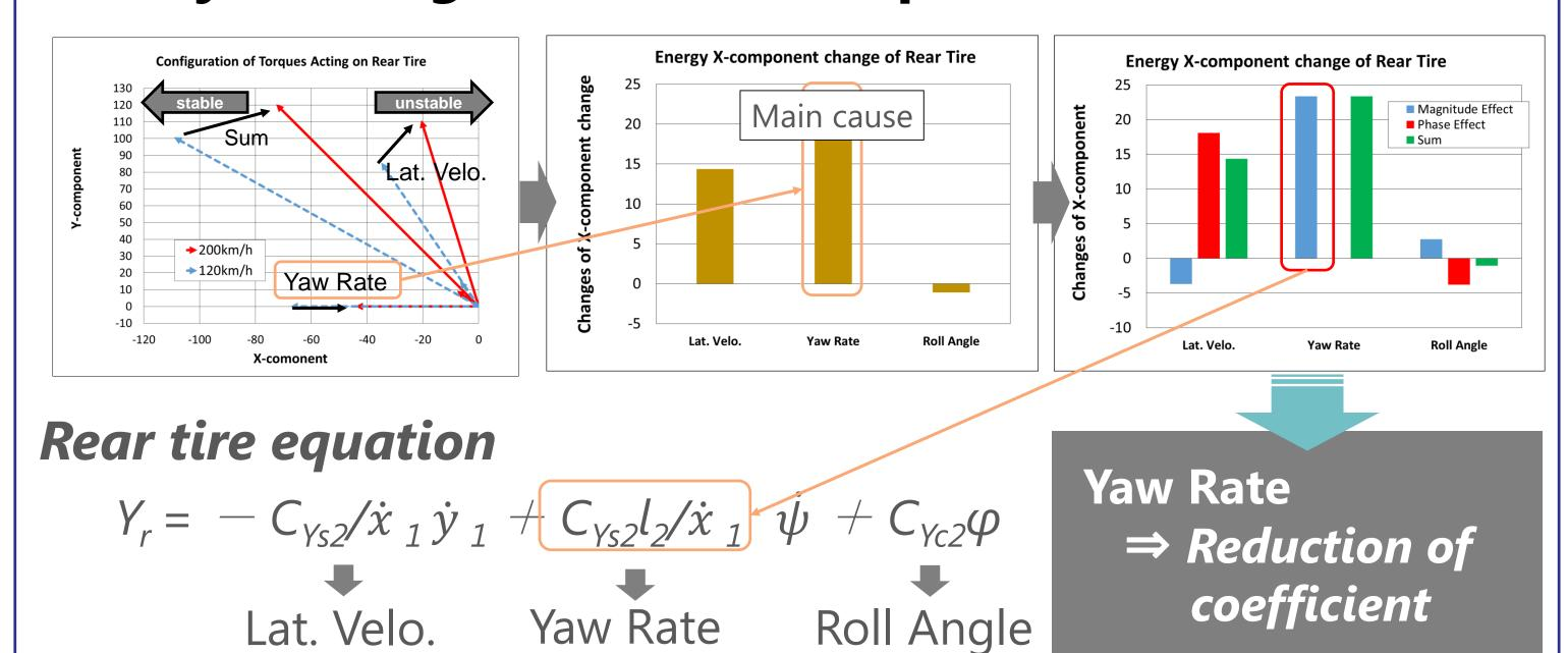
The cause is  $C_{y_{s2}}$  or  $\dot{x}_1$
