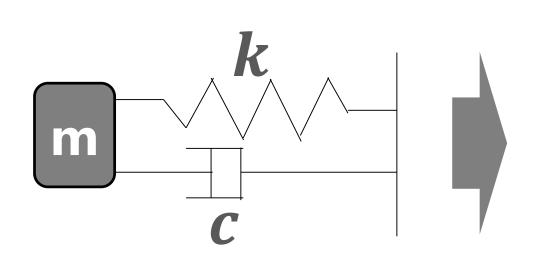
Equation of motion  $m\ddot{x} + c\dot{x} + kx = 0$ Eigenvalue
