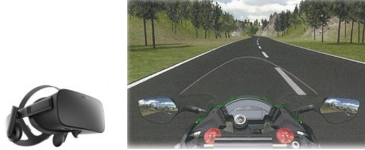
Figure 8 VR system for reproducing sense of speed.
