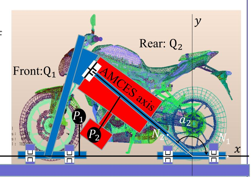
The front body (blue:  $Q_1$ ) and the rear body(red:  $Q_2$ ) are rotated using the actuators (white) at the ends of the AMCES axis. This structure acts as an inverted double pendulum, with the portion linking  $Q_1$  and  $Q_2$  dubbed Acrobot due to the placement of the actuators. The  $Q_1$  roll angle is defined as  $q_1$ , and the  $Q_2$  rotation angle as  $q_2$ .
